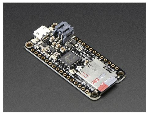
At the Feather M0's heart is an ATSAMD21G18 ARM Cortex M0 processor, clocked at 48 MHz and at 3.3V
